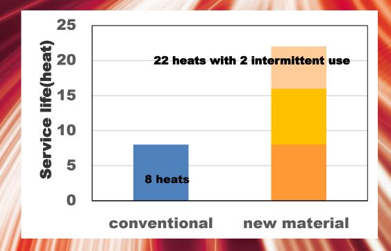
SHINAGAWA have developed long service-life ladle shroud. It is consisted of silica-free body material outside with superior erosion resistance and carbon-free liner inside with good spalling resistance. You can use them for cold start and hot start, and also continuous and intermittent use. They have performed very well and reached to over twenty heats with two-times intermittent use, which covers three tundishes.
